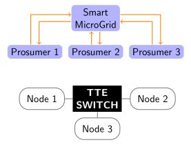
Logical architecture = information flow to ensure Providing a mapping: Smart MicroGrid  $\mapsto$  Node 2 Prosumer 1  $\mapsto$  Node 1 Prosumer 2  $\mapsto$  Node 3 Prosumer 3  $\mapsto$  Node 3
