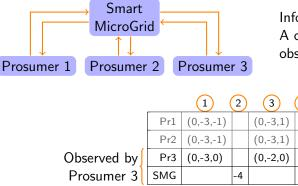
Information flow ensures that: A component can only observe its inputs and outputs
